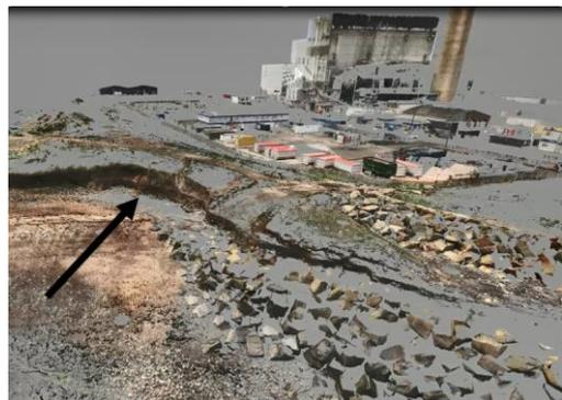
Figure 2 – 3D terrestrial laserscan survey of eroding colliery spoil at terminal end of rock revetment in Lynemouth Bay (courtesy Academy Geomatics)
